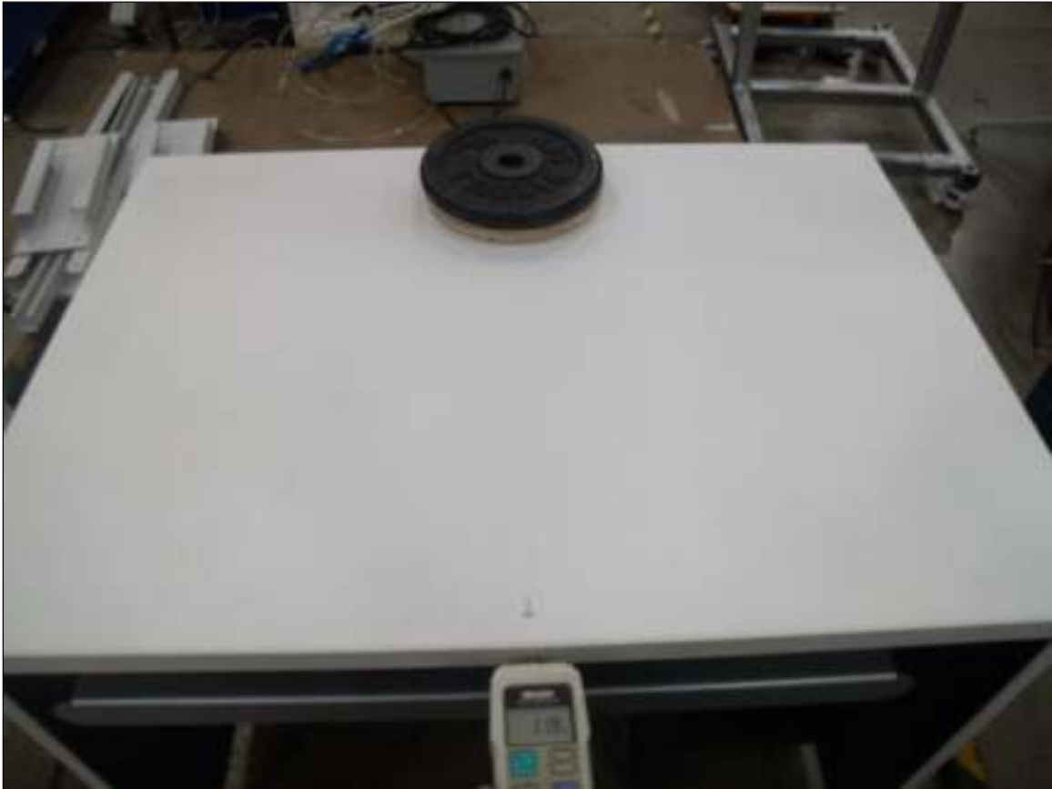
Stability Test for Keyboard/Laptop Tables (with and without casters)
