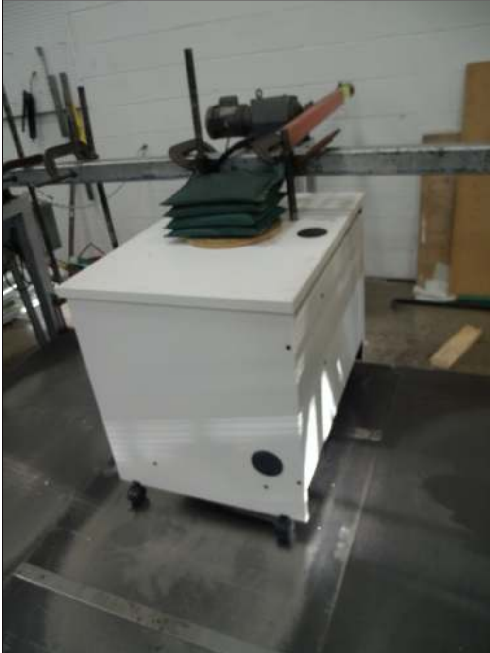
Durability Test for Desks & Tables with Casters
