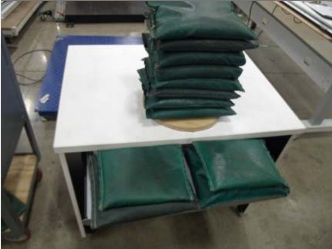
Concentrated Functional Load Test
