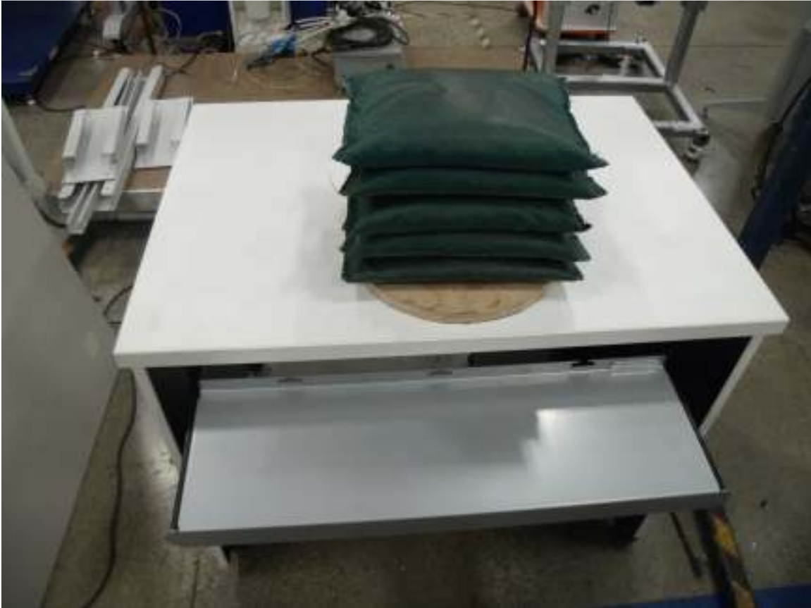
Stability Under Vertical Load Test
