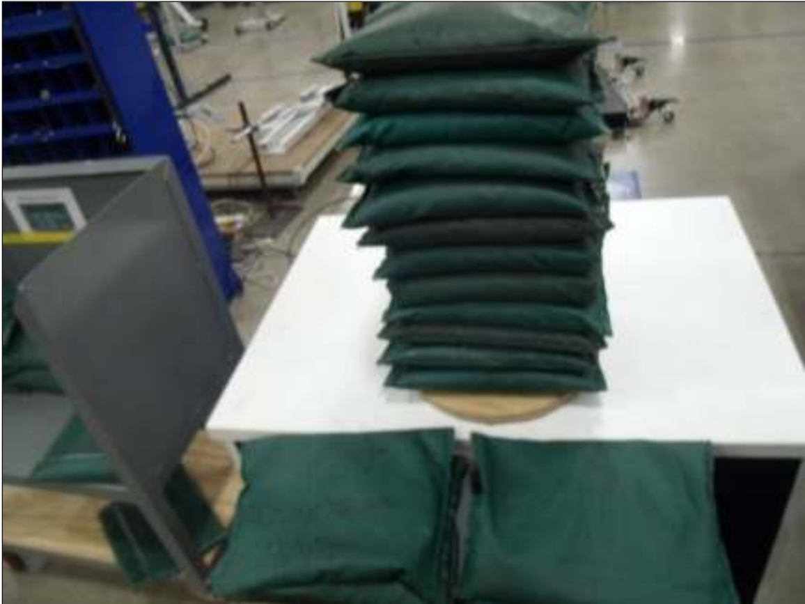
Concentrated Proof Load Test
