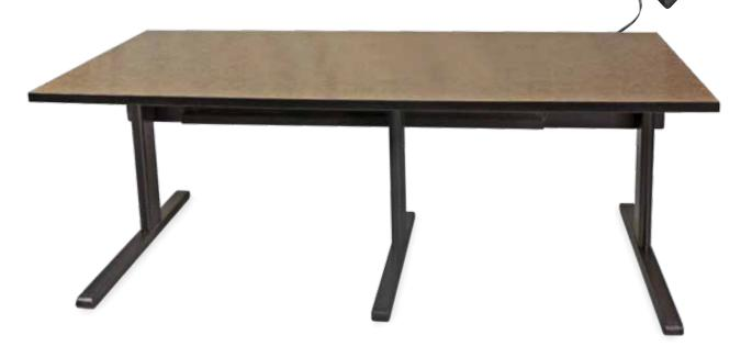
Legs are black, offset-T shaped, steel construction with wire management holes (1.5" x 4" racetrack column in 13 gauge steel, 1.5" x 2" rectangular main bar in 11 gauge steel, black nylon bullnose end caps, wire management door optional add-on), 1" diameter levelers
