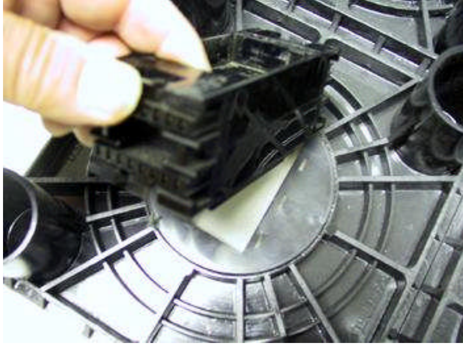
Picture 9-8 Installing Powerport Clips
