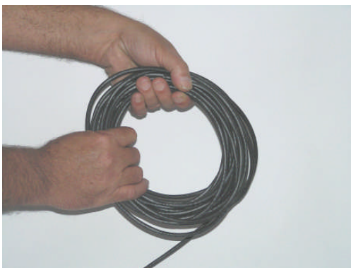
Correct !!! Hand over hand unrolling out.
