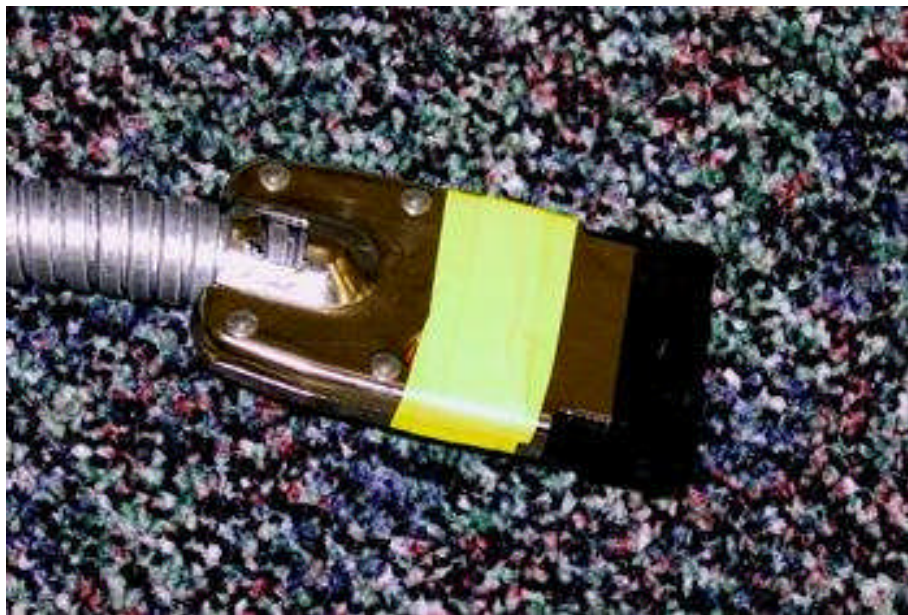
Picture 9-15 Completed Color Coding of Cable Assembly
