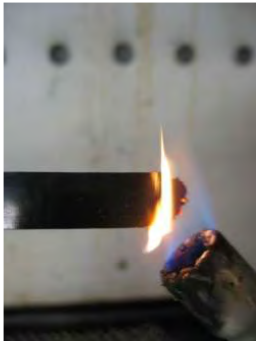
Photo No. 20 ASTM D 635 - Flame Exposure Detail
