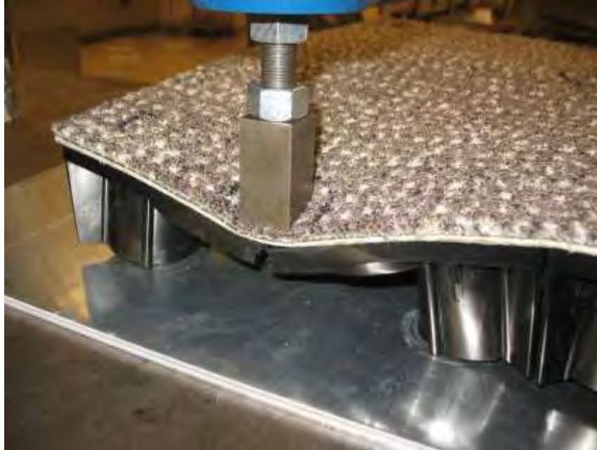
Photo No. 13 CISCA Sections 1 and 2 - Quarter Panel Midpoint Edge Loading Test Panel Fracture Failure
