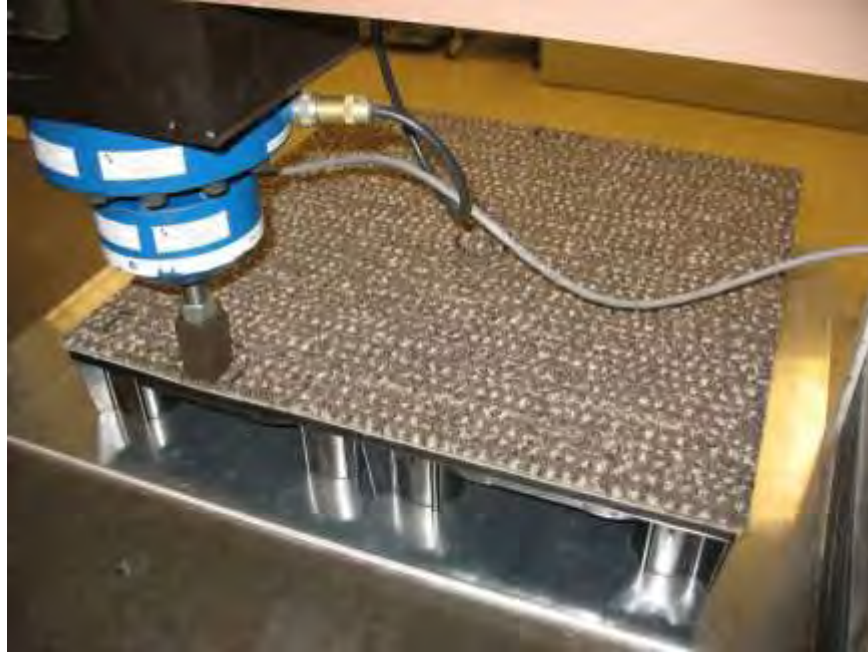
Photo No. 11 CISCA Sections 1 and 2 - Quarter Panel Midpoint Edge Loading Test Setup
