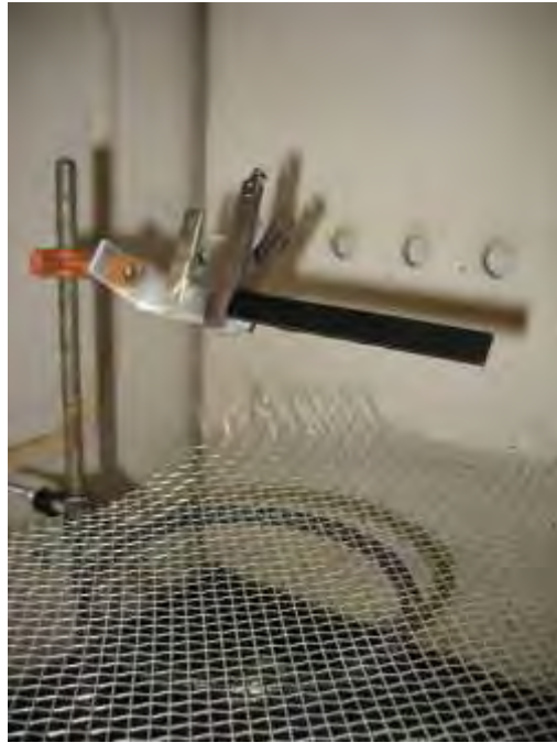
Photo No. 19 ASTM D 635 - Rate of Burn Test Setup
