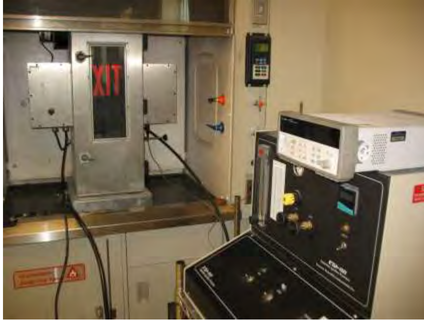
Photo No. 25 ASTM D 2643 - Smoke Density Test Apparatus
