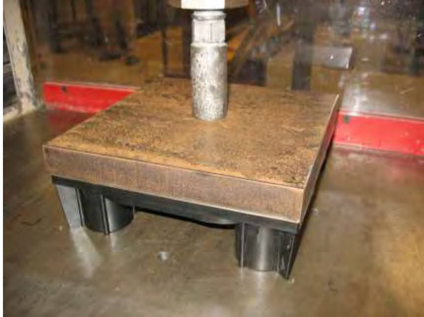
Photo No. 29 Full Panel Load Bearing Area Failure Load Evaluation Test Setup
