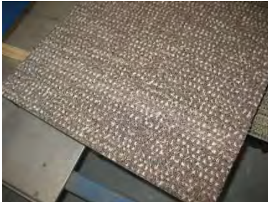
Photo No. 16 CISCA Section 3 - Travel Path 2 (Quarter Panel Center) Post-Cycling Specimen Condition
