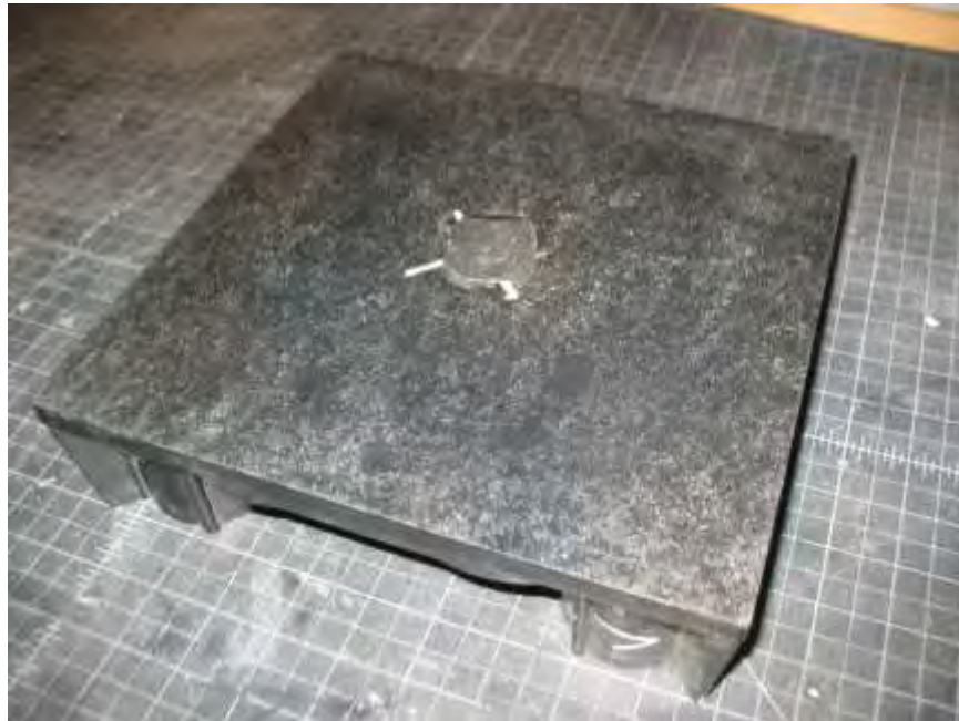
Photo No. 28 ASTM E 2322 - Typical Posttest Condition Uniform Load Specimen (No Damage Observed Post 1,600 psf Applied Load)
