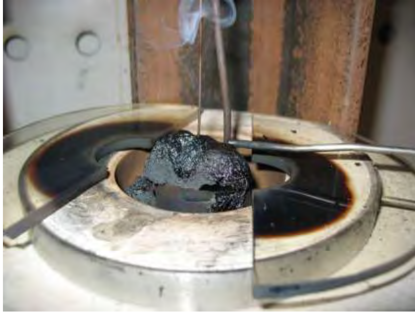
Photo No. 23 ASTM D 1929 - Typical Post-Ignition Specimen Condition
