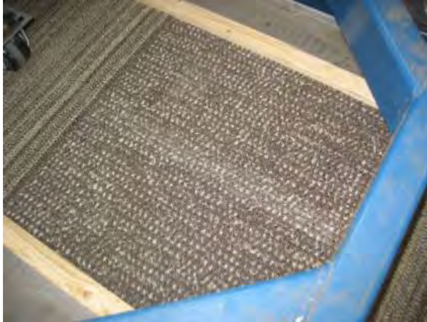
Photo No. 15 CISCA Section 3 - Travel Path 1 (Full Panel Center) Post-Cycling Specimen Condition
