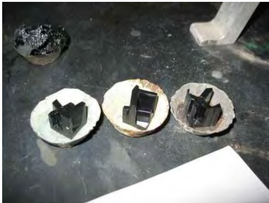
Photo No. 22 ASTM D 1929 - Typical Pretest Condition Ignition Specimens
