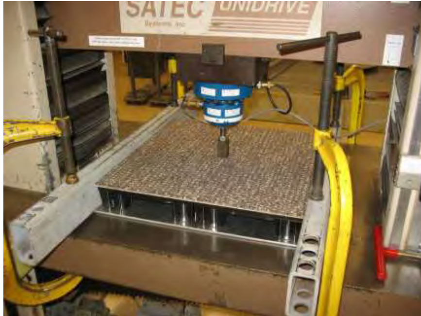
Photo No. 3 CISCA Sections 1 and 2 - Full Panel Center Point Loading Test Setup
