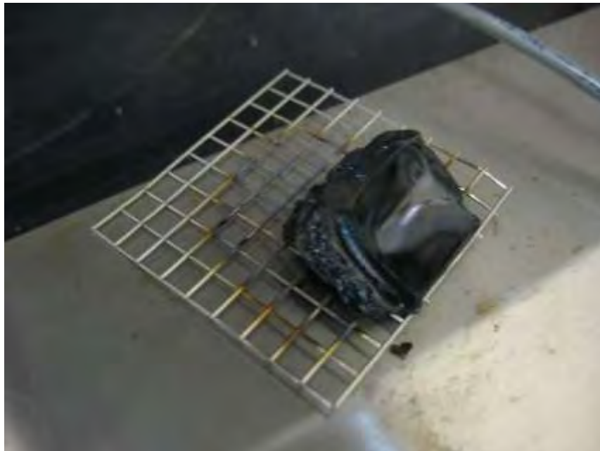
Photo No. 26 ASTM D 2643 - Typical Post-Exposure Condition Smoke Density Specimen
