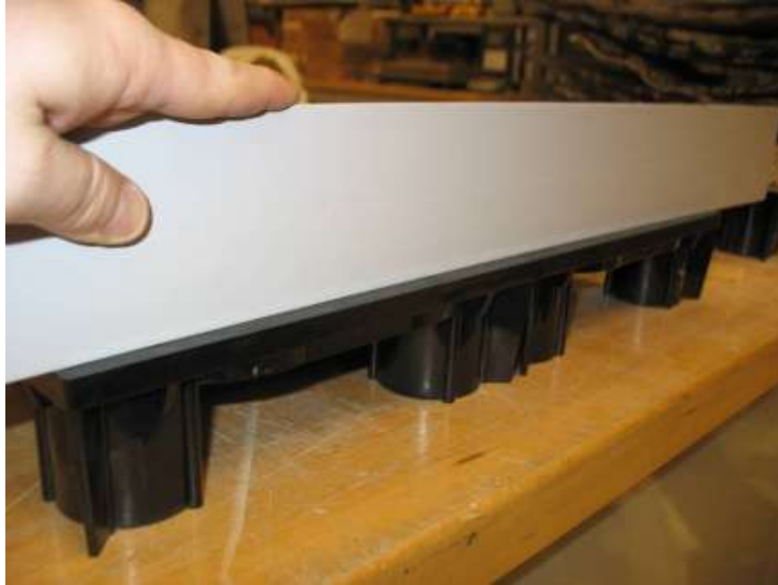
Photo No. 17 CISCA Section 3 - Post-Cycling Beam Deformation Measurement
