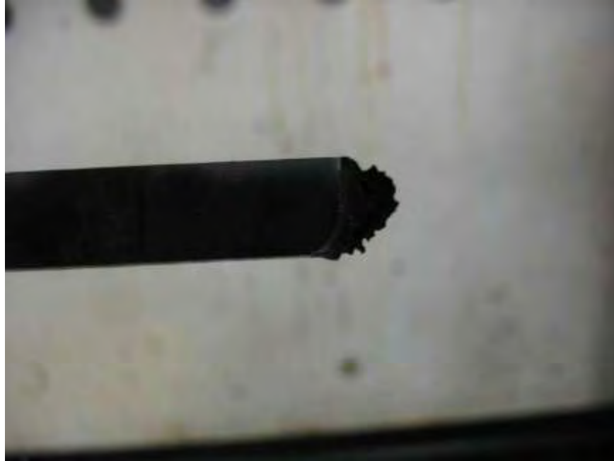
Photo No. 21 ASTM D 635 - Typical Post Exposure Specimen Detail
