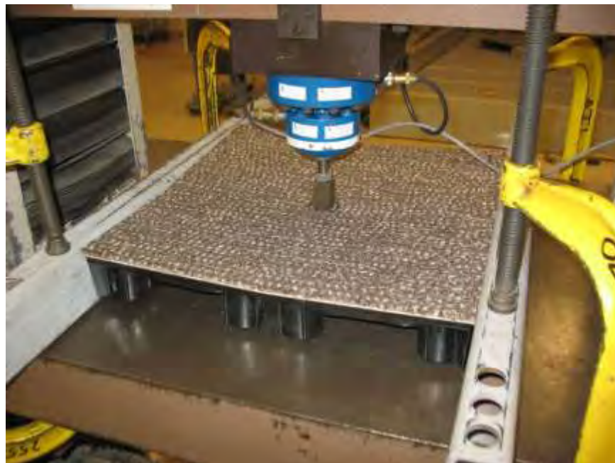
Photo No. 4 CISCA Sections 1 and 2 - Full Panel Center Point Loading Test in Progress
