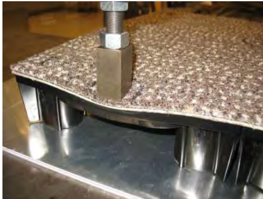
Photo No. 12 CISCA Sections 1 and 2 - Quarter Panel Midpoint Edge Loading Test in Progress
