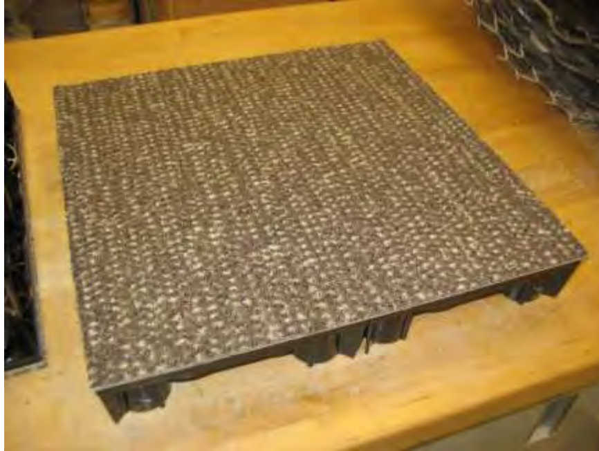
Photo No. 1 Typical Fixed Height Low Profile Raised Floor System Panel Specimens As-Received
