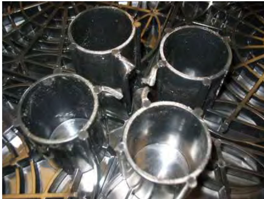
Photo No. 6 CISCA Sections 1 and 2 - Full Panel Center Point Loading Test Underside Failure Detail
