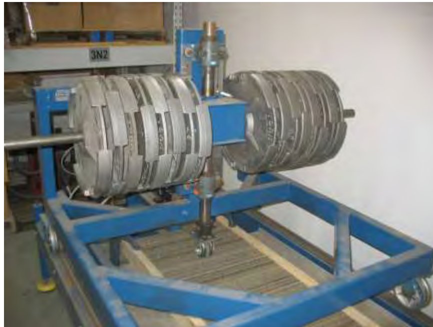
Photo No. 14 CISCA Section 3 - Rolling Load Test Apparatus
