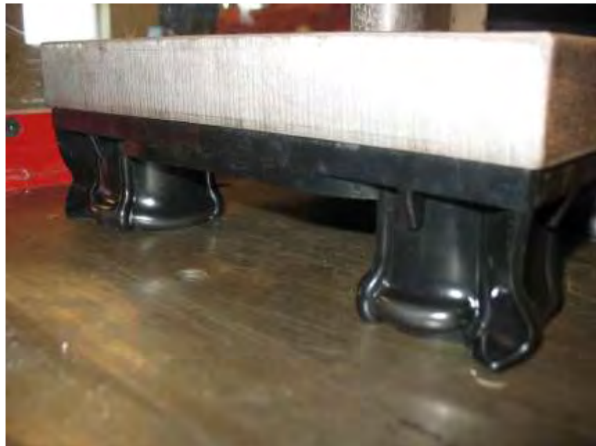
Photo No. 30 Typical Full Panel Load Bearing Area Failure Load Evaluation Compressive Failure Detail
