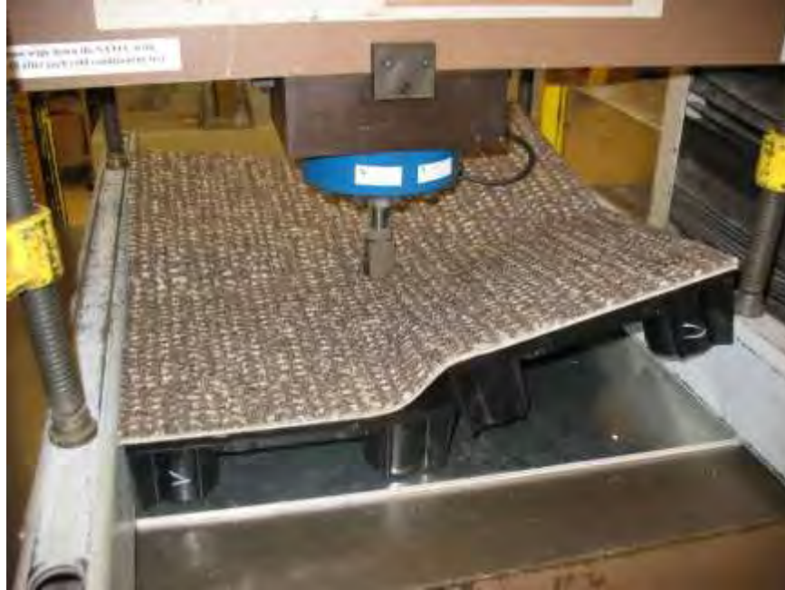
Photo No. 5 CISCA Sections 1 and 2 - Full Panel Center Point Loading Test Kick Out Failure
