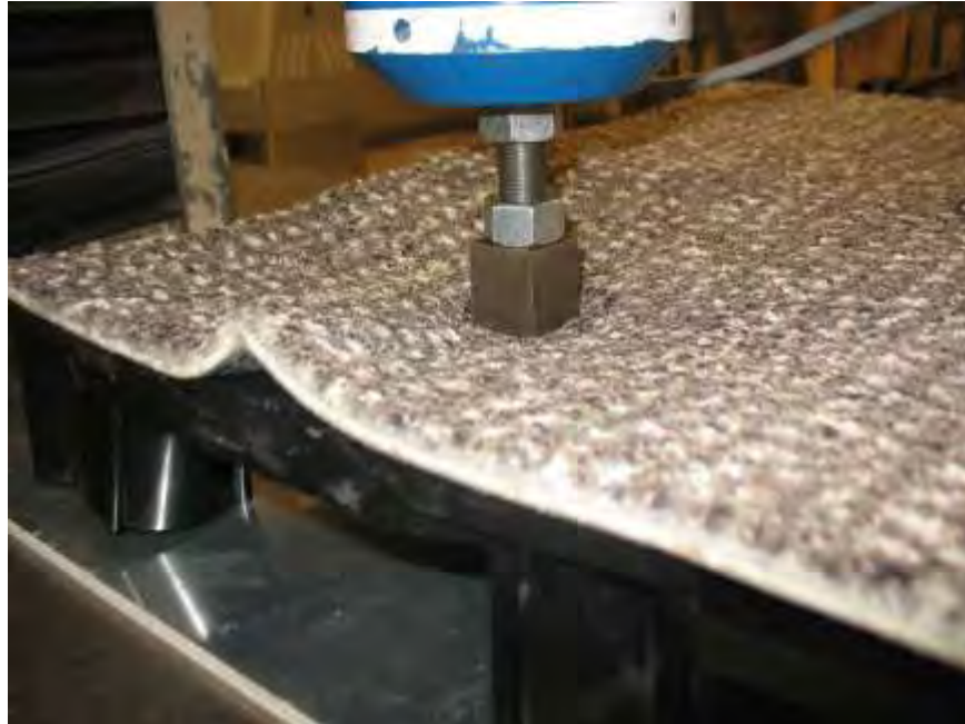
Photo No. 9 CISCA Sections 1 and 2 - Center of Quarter Panel Loading Test Panel Fracture Failure
