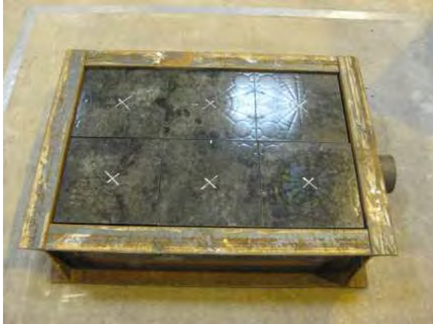
Photo No. 27 ASTM E 2322 - Uniform Load Evaluation Test Fixture
