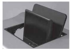
Increase the angle by holding the lid with one hand and the top of the display with the other, then bring the display toward you.
