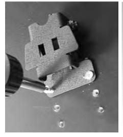
The male half of the VESA mount is attached to the flipIT lid with three Euroscrews. Additional mounting locations, at half-inch intervals, are
