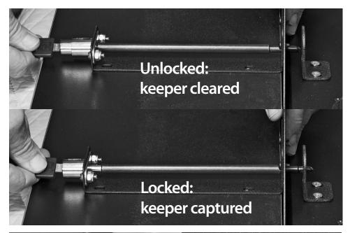
Loosen the keeper Euro screws and slide it so that it clears the the plunge lock bar in the unlocked position.
