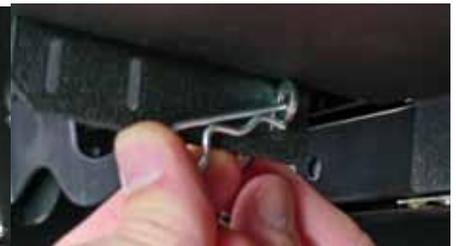
Fit cable ends through slots provided in the keyboard tray, then secure the ends with beta pins.
