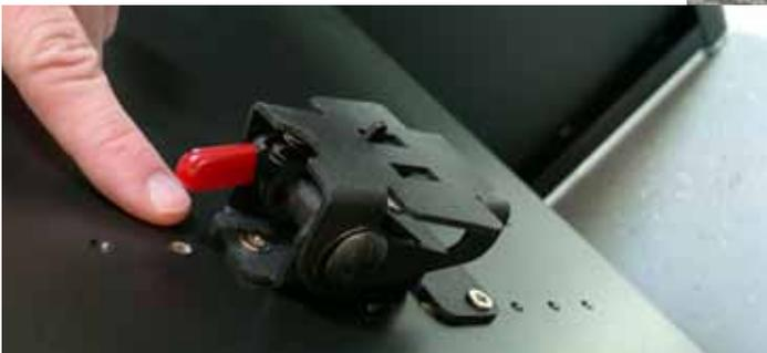
Monitor bracket may be repositioned, if needed, to achieve 1/2" maximum clearance between the monitor top and the lid rest. Mounting positions are provided in 1/2" increments.
