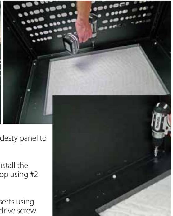
Flex the loosely installed base panels to permit capture of the machine screws by the modesty panel.
