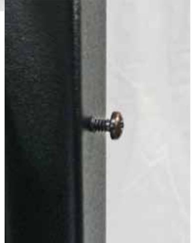
Position base panels over inserts with wire management holes on the modesty panel side. Use 1/4-20 hex head /#2 Phillips drive bolts to loosely install the base panels; three for each panel. (See below, as to why the bolts are installed only about half way).
