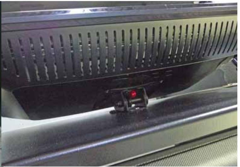
The VESA mounting bracket is in two pieces that nest together when installed. The bracket ships attached to the lid and is secured with a cable tie. Remove the cable tie and affix the bracket onto the monitor using holes 100mm or 75mm square: the VESA standard. Use the 6mm screws that come with the monitor.
