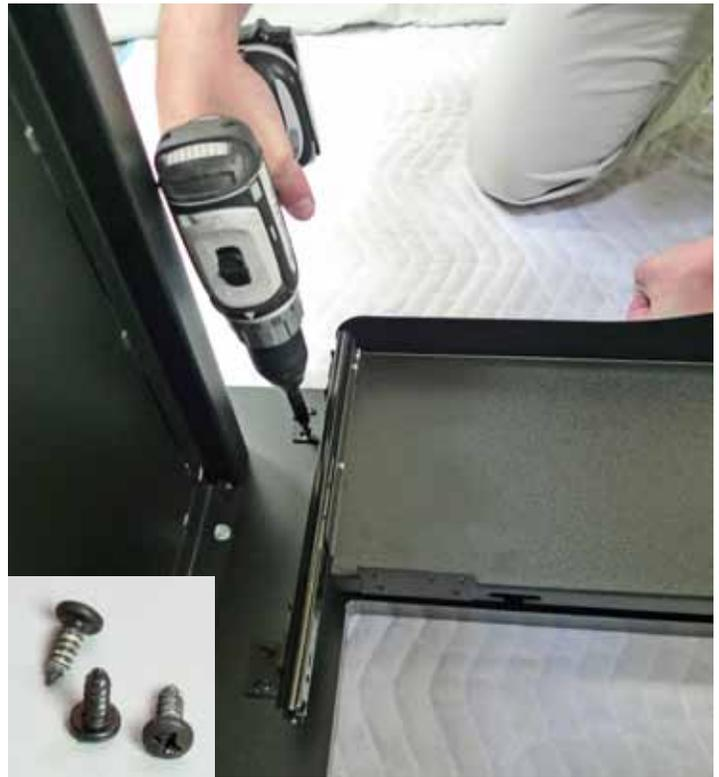
Eight #2 Phillips drive wood screws are provided with the flipIT Kit for installing the keyboard tray.
