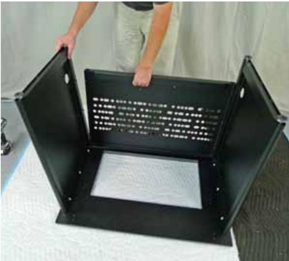
Flex the loosely installed base panels to permit capture of the machine screws by the modesty panel.
