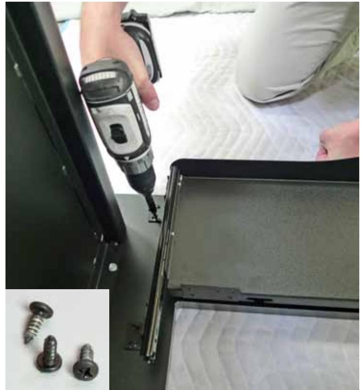
Eight #2 Phillips drive wood screws are provided with the flipIT Kit for installing the keyboard tray.
