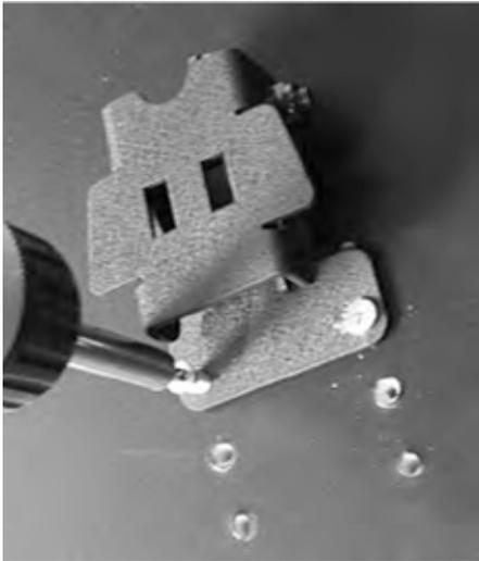
The male half of the VESA mount is attached to the flipIT lid with three Euro screws. Additional mounting locations, at half-inch intervals, are provided to fine-tune the
