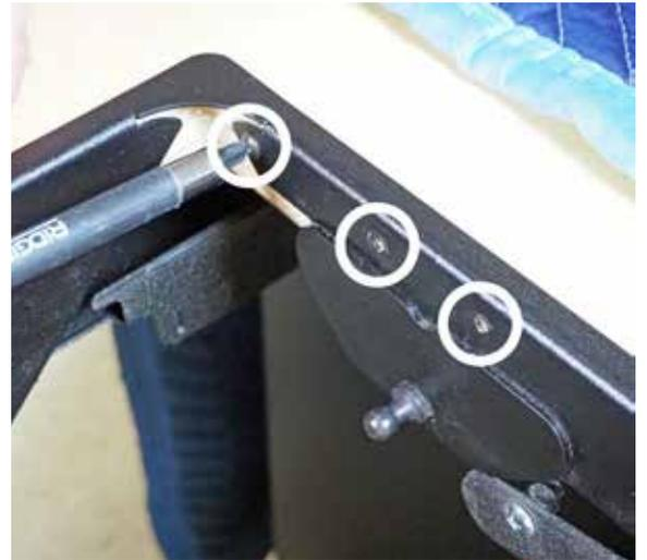
Lift the lid open all the way and complete the installation. One screw installs the right side corner. 3 screws reinforce the gas spring mounting post location on the left side.
