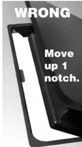
balance of the opening performance. If the monitor is mounted too high, it will not pass through the cutout.
