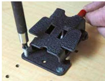
There are 6 sets of mounting holes spaced 1/2" apart to choose from. Mount the bracket in the 3rd one and see if it works with your display. If it needs to be moved, choose the best location. Install with 3 Euro-screws.
