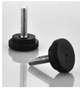
Floor Glides, 2 per panel. 1" diameter x 1" adjustment, 1/4" x 20 thread.
