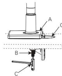
CAUTION: Clamp Mounts cannot be used to mount the M8 to any vertical surface.
