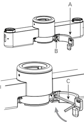
**CAUTION:** If the lever is difficult to close or will not close fully, it is over-tightened. Turn the Adjustment screw counter-clockwise slightly. Forcing it closed will cause damage to MFlex.
