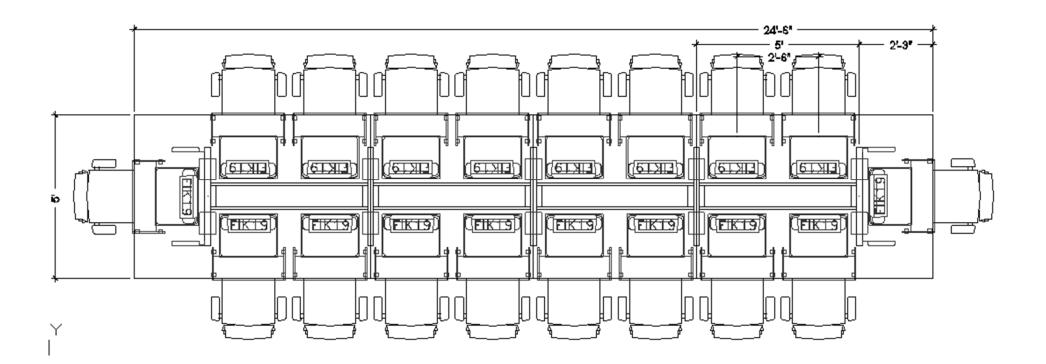
The table above can include any of the following: FIK19, FIH19 or FIL18. Drawing shows the maximum number of flipITs. FlipITs may be eliminated from any or all locations shown.
