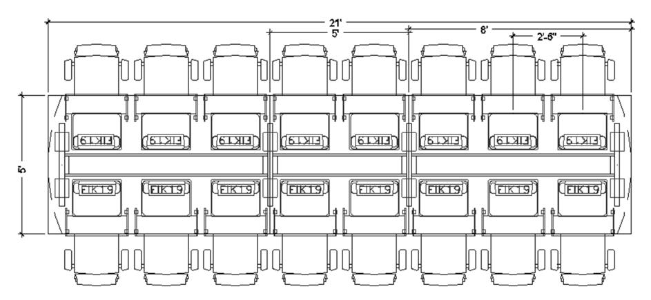
The table above can include any of the following: FIK19, FIH19 or FIL18. Drawing shows the maximum number of flipITs. FlipITs may be eliminated from any or all locations shown.
