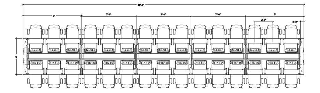
The table above can include any of the following: FIK19, FIH19 or FIL18. Drawing shows the maximum number of flipITs. FlipITs may be eliminated from any or all locations shown.
