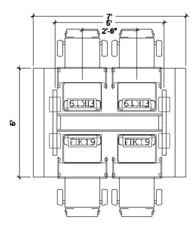
The table above can include any of the following: FIK19, FIH19 or FIL18. Drawing shows the maximum number of flipITs. FlipITs may be eliminated from any or all locations shown.
