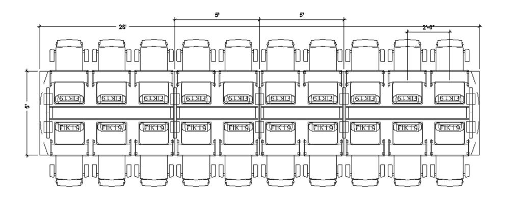
The table above can include any of the following: FIK19, FIH19 or FIL18. Drawing shows the maximum number of flipITs. FlipITs may be eliminated from any or all locations shown.
