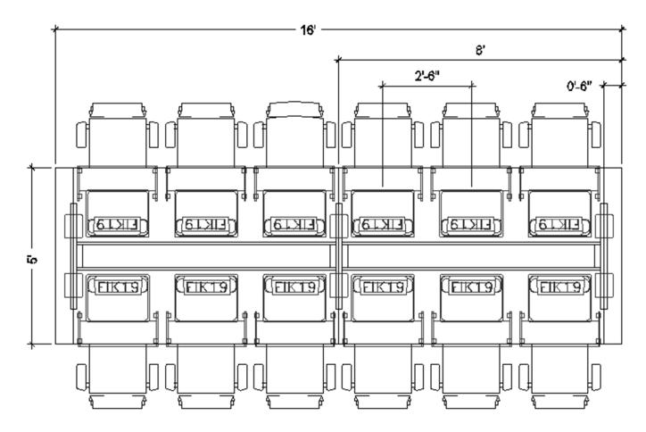
The table above can include any of the following: FIK19, FIH19 or FIL18. Drawing shows the maximum number of flipITs. FlipITs may be eliminated from any or all locations shown.
