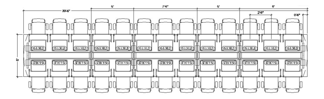
The table above can include any of the following: FIK19, FIH19 or FIL18. Drawing shows the maximum number of flipITs. FlipITs may be eliminated from any or all locations shown.
