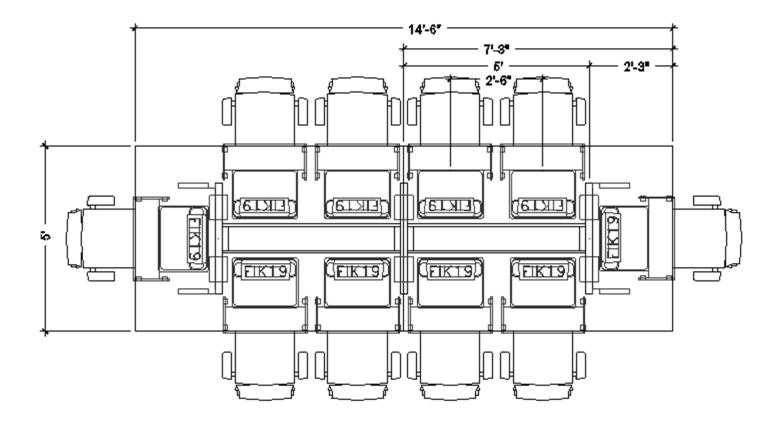
The table above can include any of the following: FIK19, FIH19 or FIL18. Drawing shows the maximum number of flipITs. FlipITs may be eliminated from any or all locations shown.
