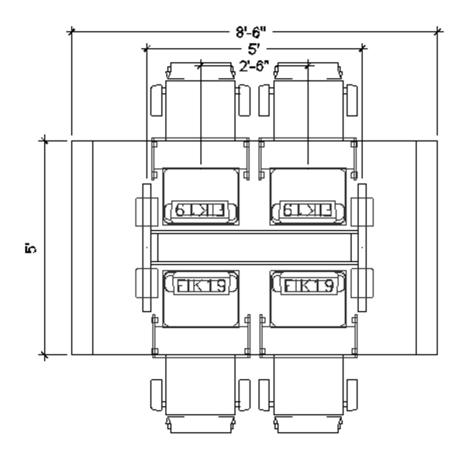
The table above can include any of the following: FIK19, FIH19 or FIL18. Drawing shows the maximum number of flipITs. FlipITs may be eliminated from any or all locations shown.
