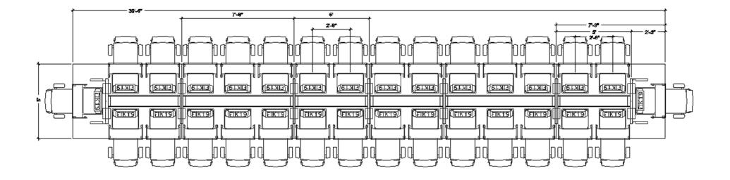
The table above can include any of the following: FIK19, FIH19 or FIL18. Drawing shows the maximum number of flipITs. FlipITs may be eliminated from any or all locations shown.
