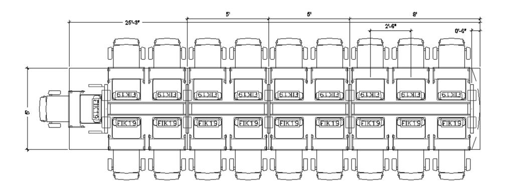
The table above can include any of the following: FIK19, FIH19 or FIL18. Drawing shows the maximum number of flipITs. FlipITs may be eliminated from any or all locations shown.
