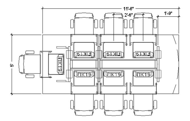
The table above can include any of the following: FIK19, FIH19 or FIL18. Drawing shows the maximum number of flipITs. FlipITs may be eliminated from any or all locations shown.
