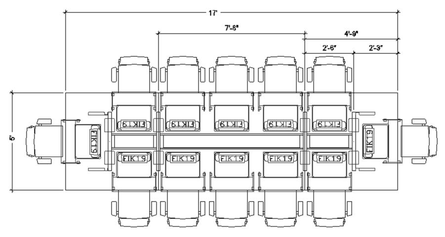
The table above can include any of the following: FIK19, FIH19 or FIL18. Drawing shows the maximum number of flipITs. FlipITs may be eliminated from any or all locations shown.
