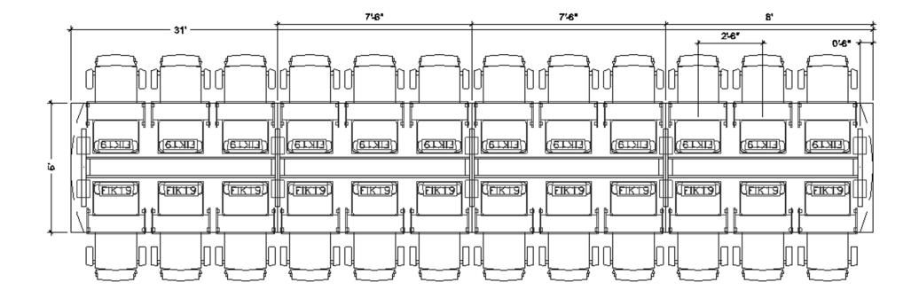
The table above can include any of the following: FIK19, FIH19 or FIL18. Drawing shows the maximum number of flipITs. FlipITs may be eliminated from any or all locations shown.
