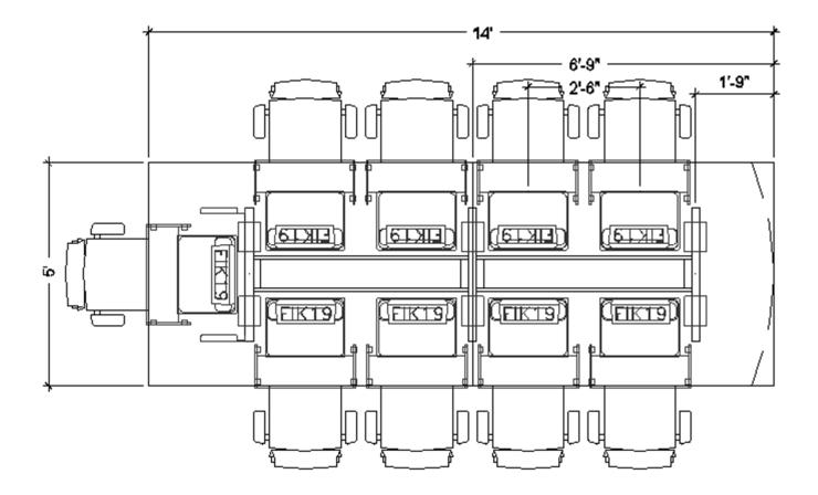
The table above can include any of the following: FIK19, FIH19 or FIL18. Drawing shows the maximum number of flipITs. FlipITs may be eliminated from any or all locations shown.
