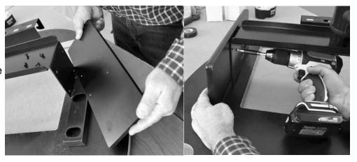
Remove the 3 hex/Phillips drive bolts that attach the bottom plate to the pedestal assembly. Keep the bolts ready for reattachment after the base plate has been installed.
