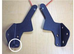
One pair (left and right) lid hinge brackets. Note the gas spring post that pairs with the post in the frame for operation. These are shipped partially assembled with bushings in the holes for the hinge pin and cables to attach to the keyboard tray or PULL handle actuator.
