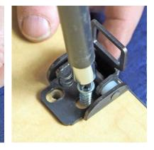
At the top of the frame, find the diagonal pilot holes at loction C. Use 2 Euro-screws to install the bracket with a screw gun and #2 Phillips driver. If your installation includes an optional Lid Lock, install it at your preference of the location D pilot holes.
