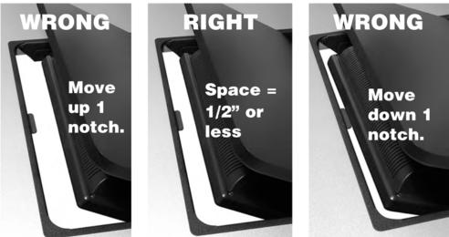
balance of the opening performance. If the monitor is mounted too high, it will not pass through the cutout. If it is mounted too low, the opening might be too fast (like jumping off a teeter totter).
