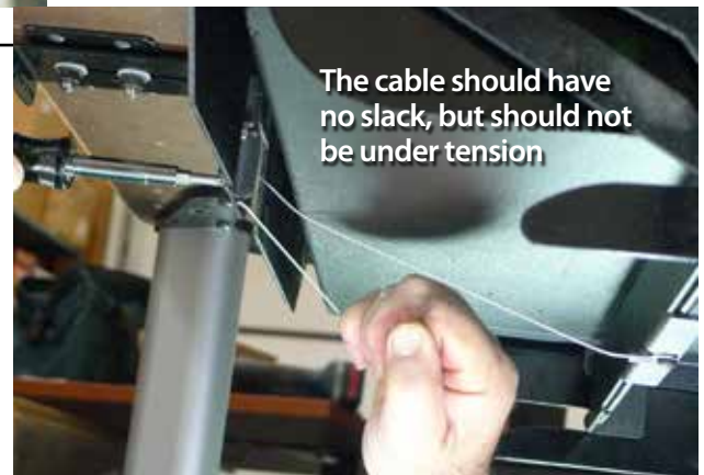
Use side cutter to trim the excess cable
