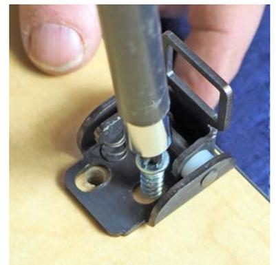
At the top of the frame, find the diagonal pilot holes at location C. Use 2 Euro-screws to install the bracket with a screw gun and #2 Phillips driver. If your installation includes an optional Lid Lock, install it at your preference of the location D pilot holes.
