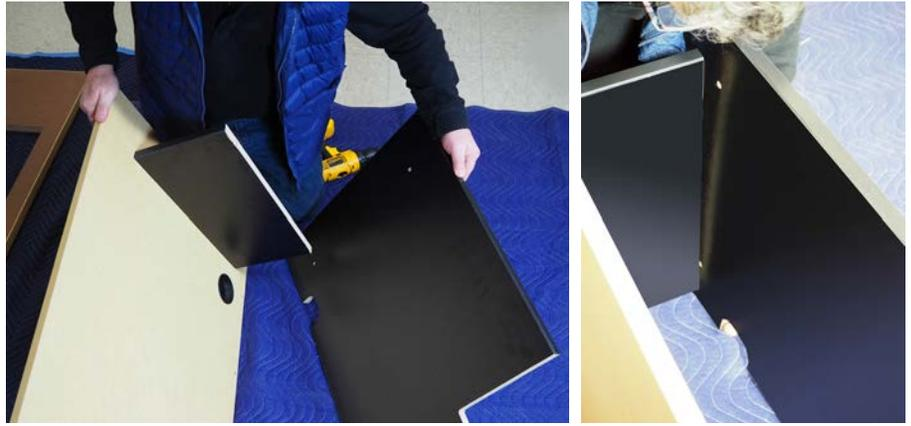
Complete the end panel CPU cabinet by securing with two Confirmats using the 4mm hex drive and screw gun.
