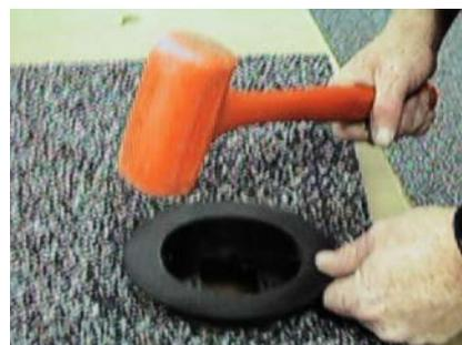
Once powerport grommet is installed into the panel, mount appropriate outlet components into the powerport and locate into the system per previous instructions.
