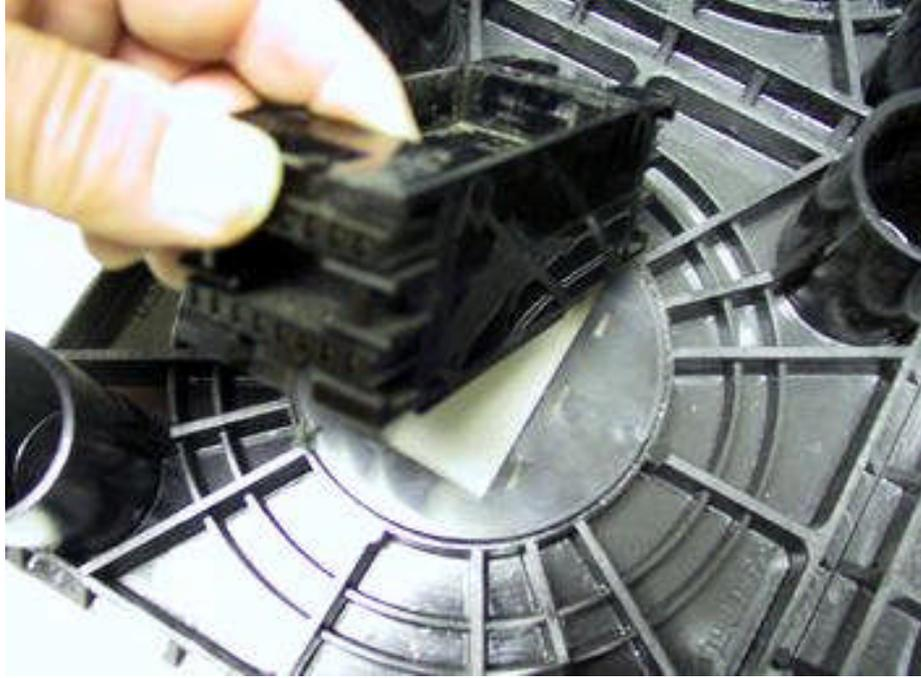
**Picture 9-8**            **Installing Powerport Clips**
