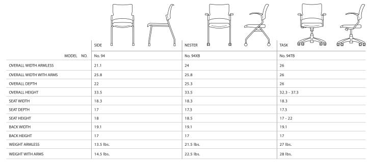
Note - For upholstered models add 1/2-inch to overall depth, 1/2-inch to seat height and 3 lbs. to weight.
