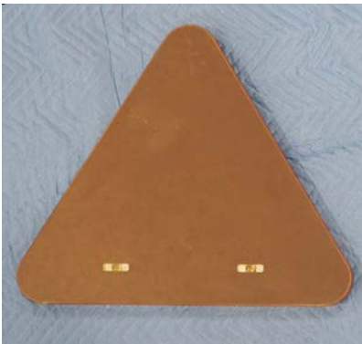
Triangular lid with milled recesses for hinges to be flush mounted.
