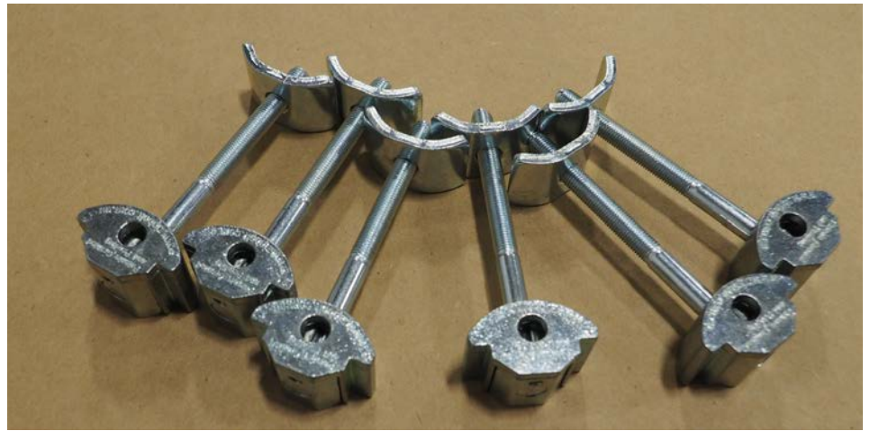
Zip bolts used to unitize the TriO top sections. Sections are fit together with spline biscuits with Zip bolts loose, tightened with 5mm hex wrench after final positioning.
