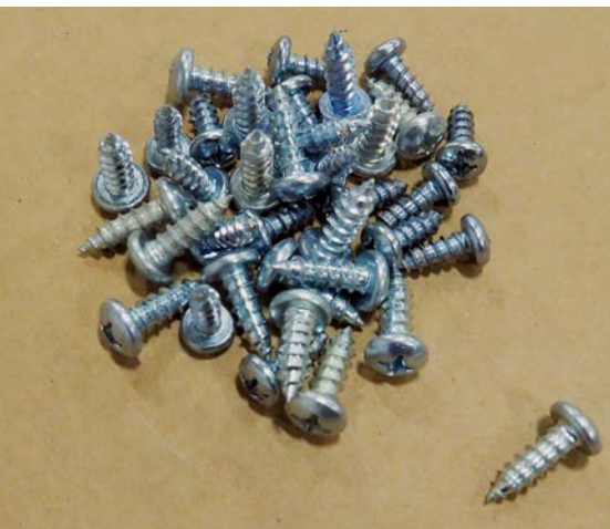
Wood screws, #10 x 3/4 pan head #2 Phillips drive, used for attaching brackets to column, top to column.
