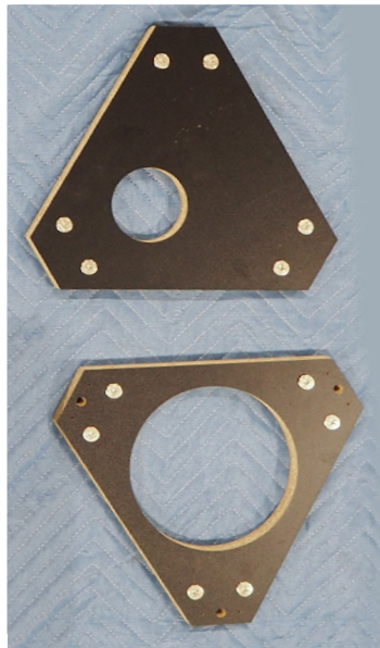
Column supports, top and bottom, with cams for pins.
